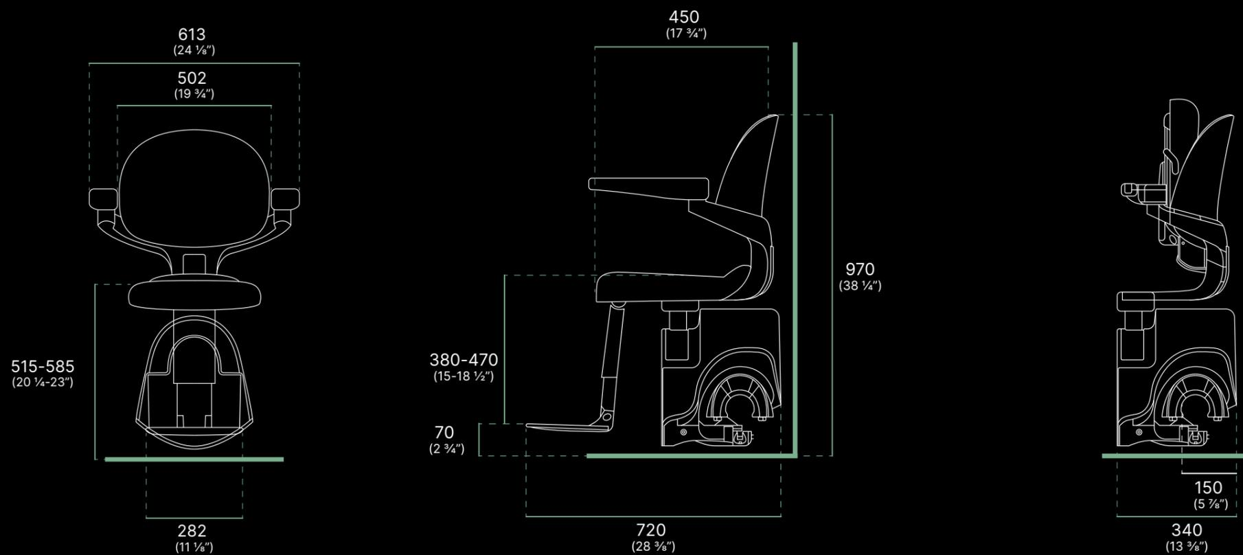
Abmessungen in mm
